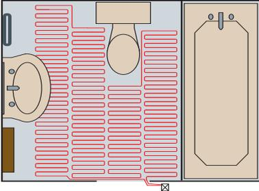
The diagram (left) shows the typical area the underfloor heating should cover.
