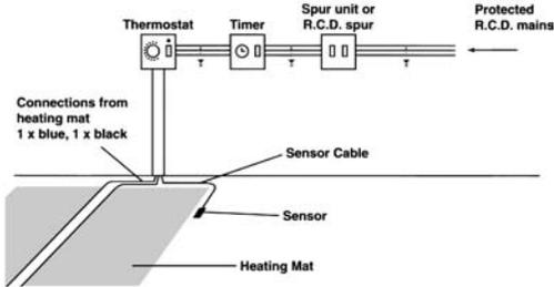
Now a qualified electrician should make the final connections in accordance with IECC guidelines. It is suggested that you use a connection box if more than one system is being connected to the device. The cold leads on the heating cables are not polarised so either can be used as positive/live, however, normal practice is to make blue positive and black negative. The cables are of co-axial construction and so have a braided earth screen running all the way through. This is a
